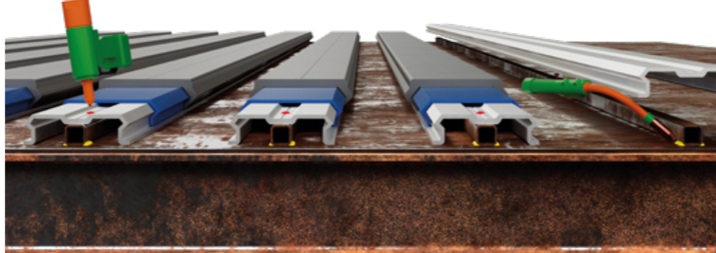
Loose aluminium subdeck profiles rivited on a steel box section welded to a steel plate.
