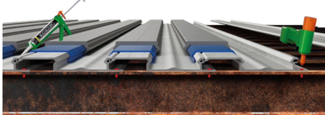
"Slide in" alu subdeck profiles rivited on steel crossmembers and sealed with sealant.
